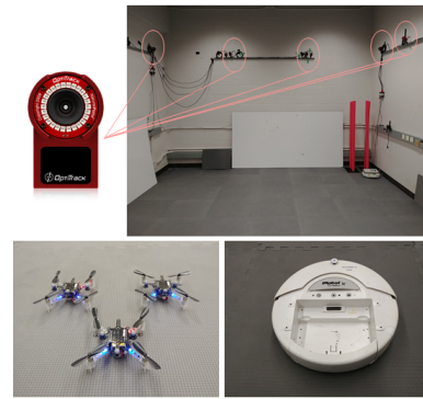
Fig. 4. Experimental Setup: Optitrack cameras in lab environment (top), Crazyflie UAVs (left), iRobot Create (right)
