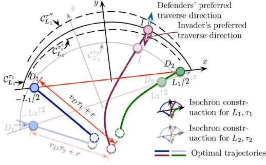
**Fig. 2.** Isochron-PEG formulation. Two groups with deep and shallow colors show two exemplar isochron constructions for different  $L, \tau$ . For fixed  $L$ , e.g.,  $L = L_1$ , different choices of  $\tau$  admit different isochrons. For  $\tau'_1 > \tau_1 > \tau''_1$ , we have  $C_{L_1}^{\tau'_1}$  above  $C_{L_1}^{\tau_1}$  above  $C_{L_1}^{\tau''_1}$ .
